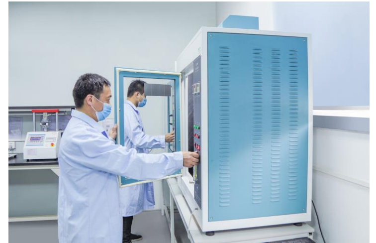
Needle Flame & Glow Wire Test
